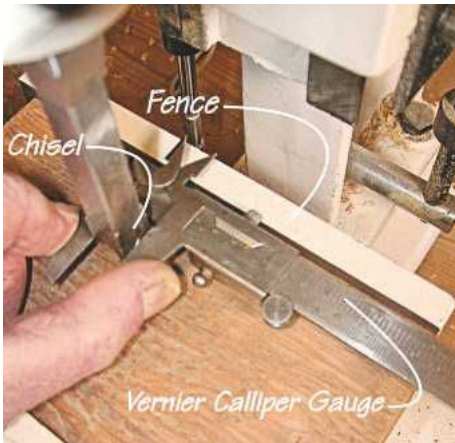
▲ Pic.5 In addition, Jeff was required to twist the chisel until the calliper's arm was parallel to the fence
